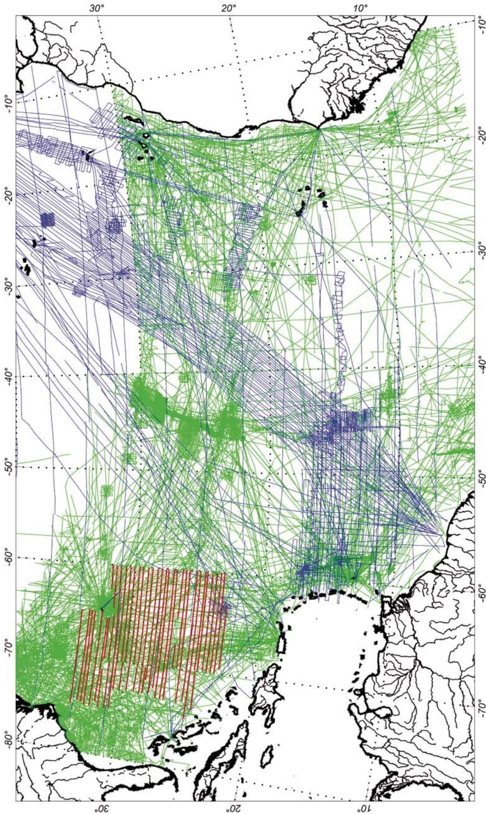
Figure 3. Magnetic anomaly profiles. GEODAS magnetic data ship-track locations (green). GSC magnetic data ship-track locations (blue) (Collette et al. 1984). Magnetic data acquired along east-west transects in 1967 and 1968 (thick red lines) (Vogt et al., 1971).
