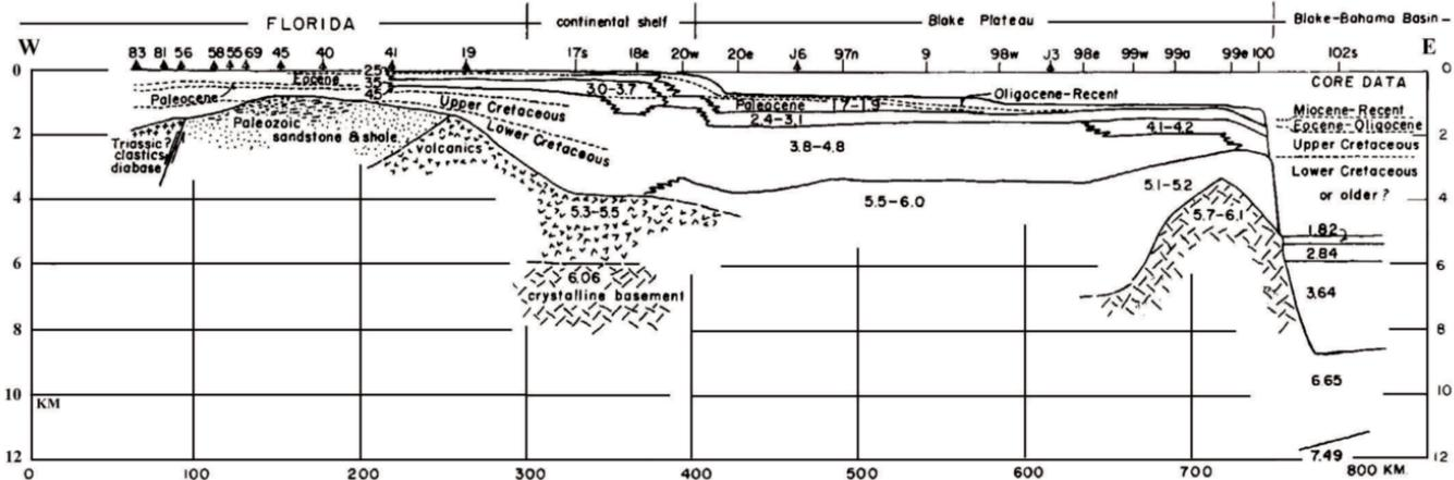
Figure 15. A west-east cross section, between  $29^\circ$  and  $30^\circ$  N across Florida and the Blake Plateau from  $84^\circ$  to  $76^\circ$  W, interpreted from seismic refraction data (Sheridan et al., 1966).
