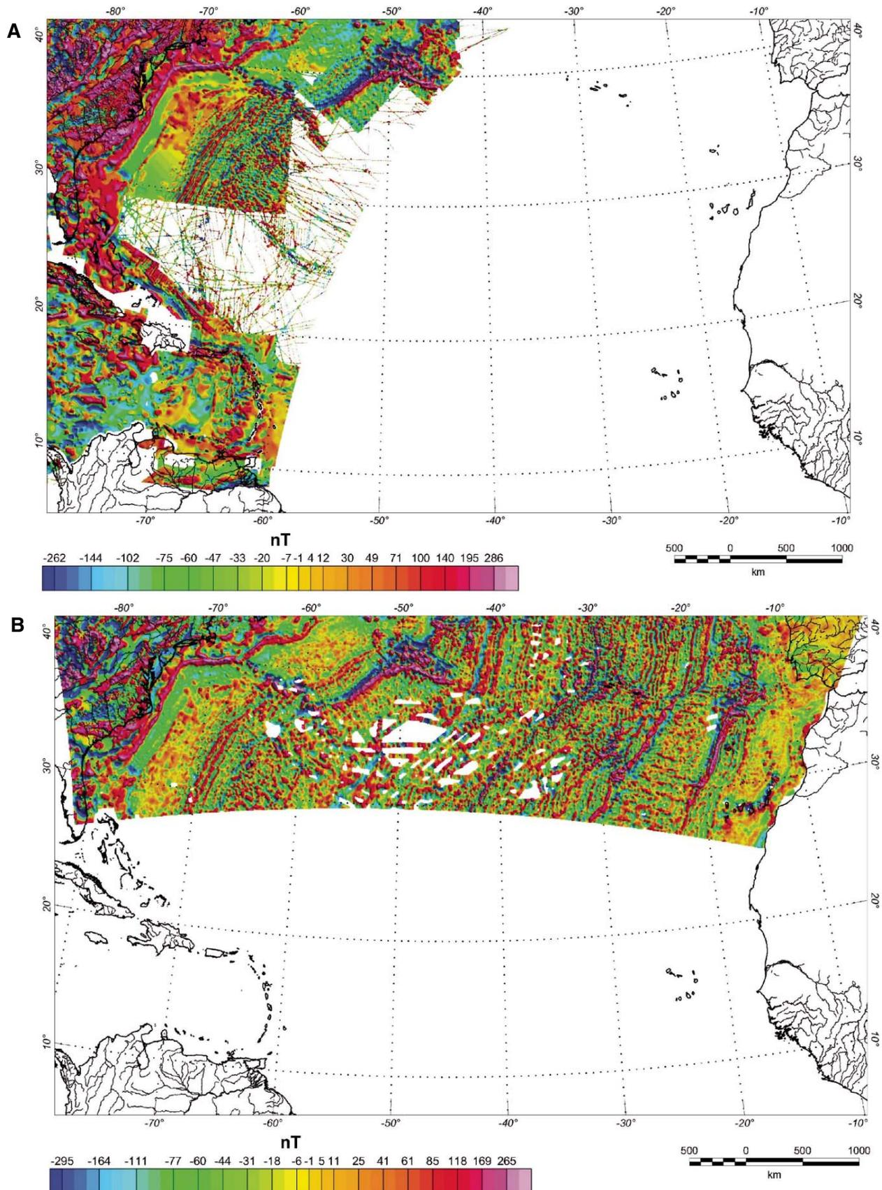
Figure 2. Magnetic anomaly grids. To the west of Chron M25 and just south of 34° N, the Geological Survey of Canada (GSC) grid is superior to the Decade of North American Geology (DNAG) grid (see Fig. 6). (A) DNAG total-intensity magnetic anomalies gridded to 2 km (Hinze et al., 1988). (B) GSC total-intensity magnetic anomalies gridded to 5 km (Verhoef et al., 1996).
